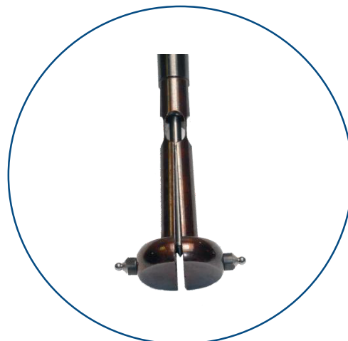
Measuring head with needle and ball inserts
