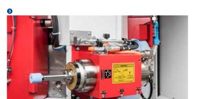
The swiveling wheelhead is equipped with water-cooled, roller-based, and maintenance-free motor spindles with stepless speed control and the latest generation of contact sensors. The shaft ends hold external wheelheads with a diameter of 500 mm (20") and a width of 63 (80 F5) mm (2.48" (3.15" F5)). For internal grinding, use powerful high-frequency spindles with 120 mm (4.72") external diameter. It's your choice: configure the wheelhead to match your specific needs.
