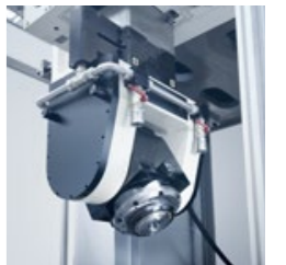
Fork grinding head Working range +/-95°.
