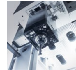
RAM with live spindle For drilling, tapping and milling operations.
