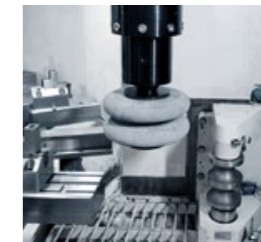
Straight grinding head RAM with live spindle is required.
