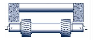
High accuracy Steering Parts can be ground in one setup with increased accuracy and efficiency.
