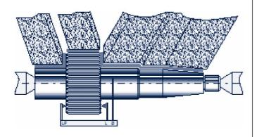
Pump Gears can be ground complete in one set-up. Form and position tolerances can be achieved much easier.
