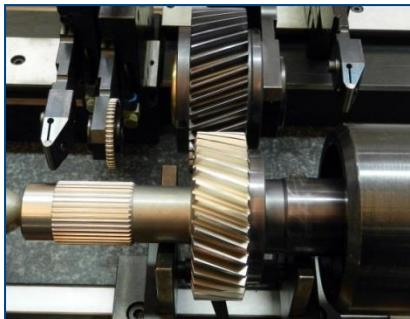
Double flank gear roll test
